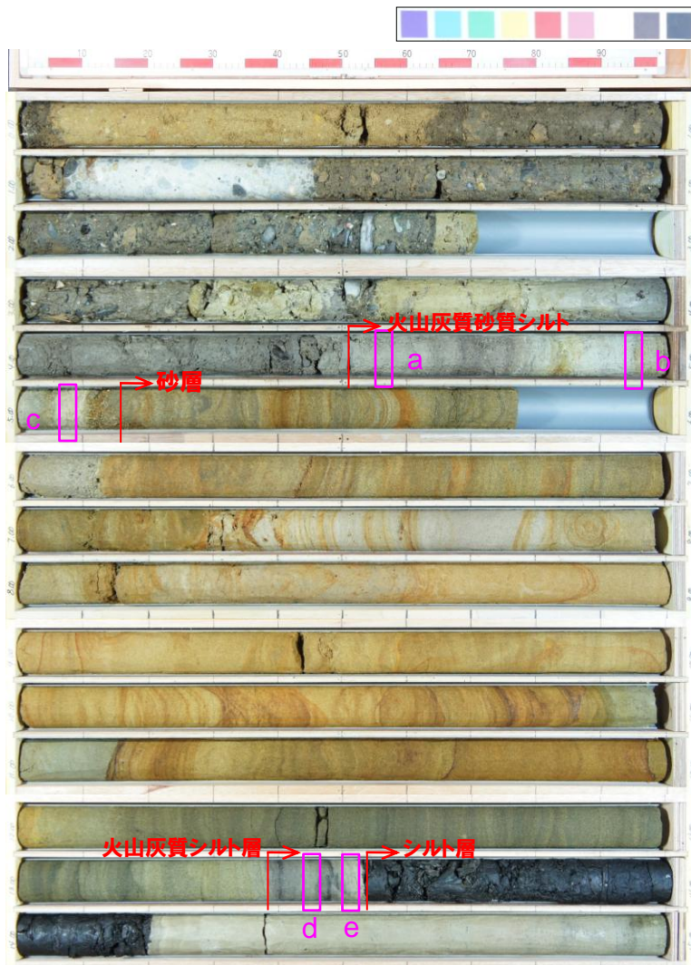
H29岩内-5コア写真(深度0~15m, 標高23.24~8.24m)
