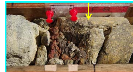
条線確認箇所拡大 (深度154.10~154.25m)
